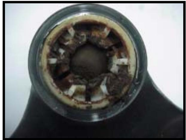
Figure 6: Remains of lubricant C on the bearing
