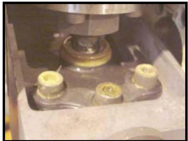
Figure 4: Test specimen in the test apparatus depicting the lack of the seal (dust cover)
