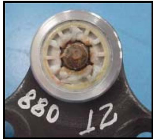
Figure 10: Lubricant A removed from test specimen 12
