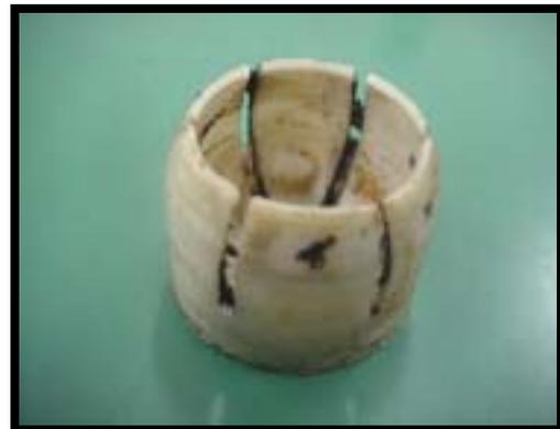
Figure 8: Plastic bearing of test specimen 02
