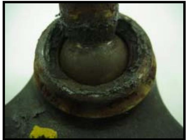
Figure 7: Loss of lubricant C on test specimen 05.
