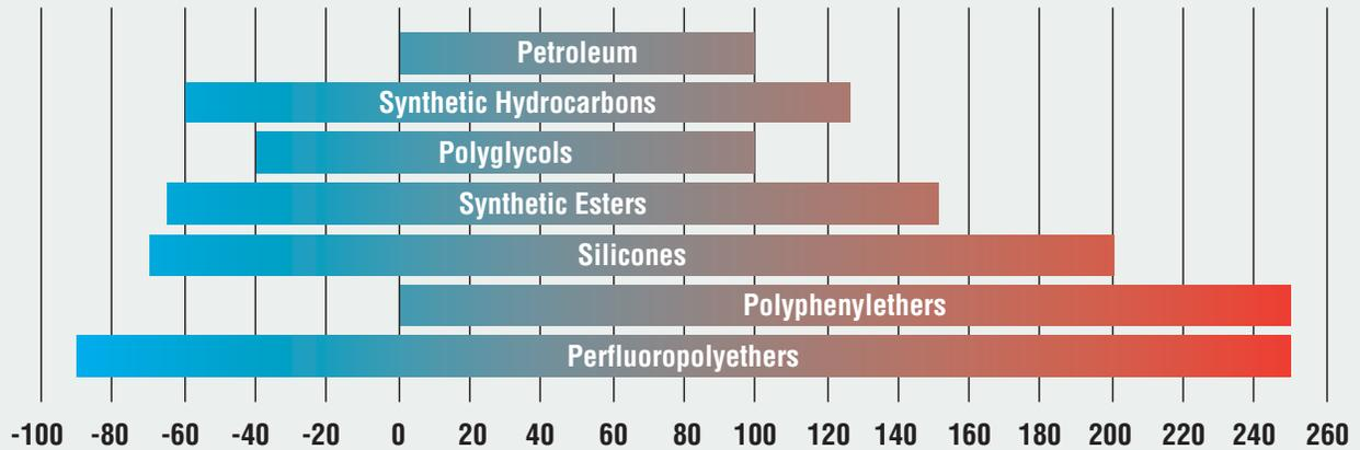
Silicones and PFPEs are compatible with nearly all gearing plastics. Both are suitable for broad temperature applications and have shown exceptional, low-temperature torque characteristics. PFPEs are also resistant to chemically aggressive environments and will not dissolve in the presence of fuel vapors or brake fluid. In addition, some PFPEs have very low vapor pressure, which is essential for vacuum chamber and aerospace applications where out gassing can be problematic.
