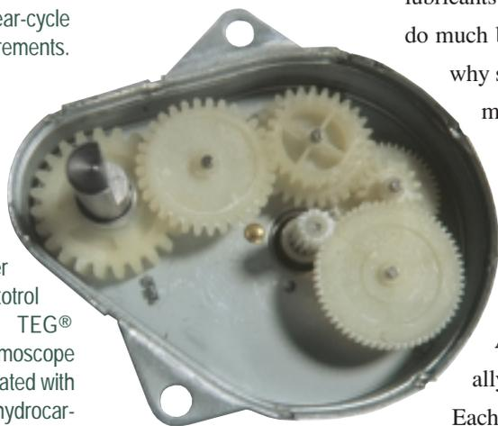
A sub-fractional horsepower electric gear motor by Autotrol Corporation powers the TEG® Coagulation Analyzer by Haemoscope Corp. Plastic gearing is lubricated with a light, thixotropic, synthetic hydrocarbon grease.
