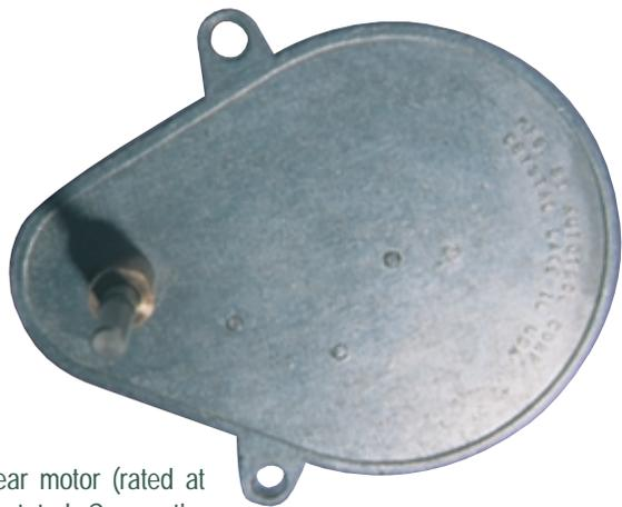
A Class N gear motor (rated at 200°C) by Autotrol Corporation uses a perfluoropolyether grease to meet its customers' 6,000 wear-cycle and 450°F temperature requirements.
