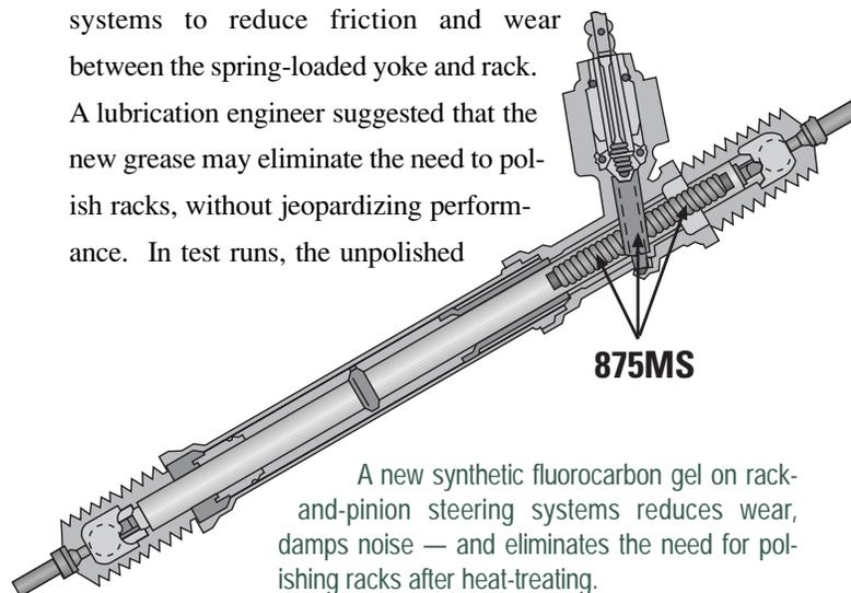
racks lubricated with the synthetic grease actually outperformed the polished units lubricated with the petroleum grease.
