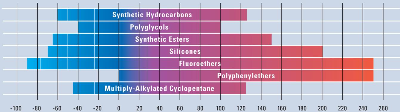
esters, at 175°C; silicones, at 200°C; and PFPEs at 250°C or higher. Most synthetics also take the cold. Polyglycols stay lubricious at -40°C; synthetic hydrocarbons, at -60°C; synthetic esters, at -65°C; silicones, at -70°C; and some PFPEs, at -90°C (See Table 1, “Lubricant Temperature Ranges”)
