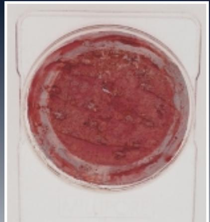
**Unfriendly skies.** Without ultrafiltration, this metal sliver would have found its way into an aircraft bearing. Metal is one of the more common contaminants found in grease.
