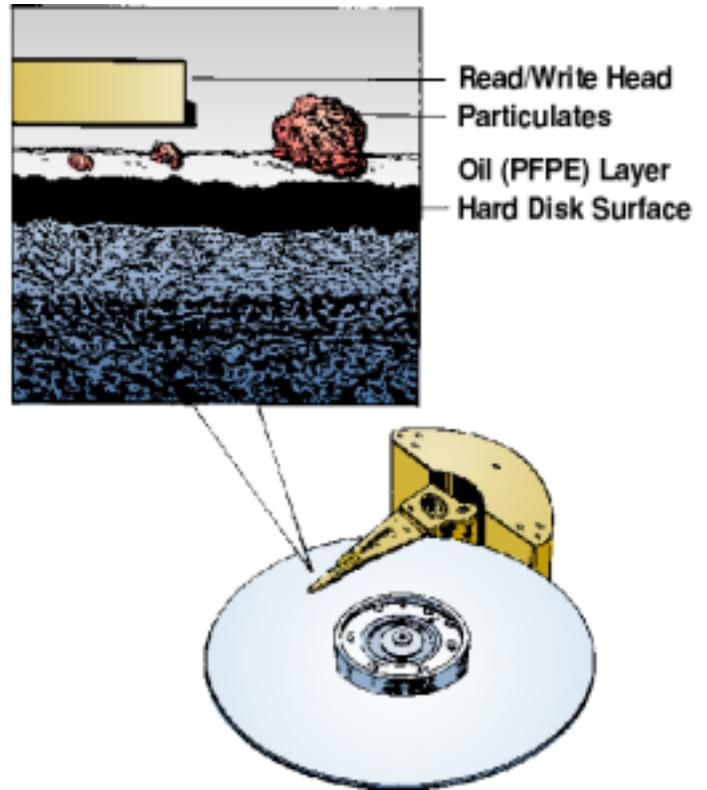
**Collision Course.** This exploded view of the head/disk surface interface shows the collision course that the head has with contamination in the film of oil that protects the disk surface. Not only are the large particles knocked around and into the surface, the smaller particles below the film surface can cause damage during the occasional bump that happens between the head and the surface layer.
