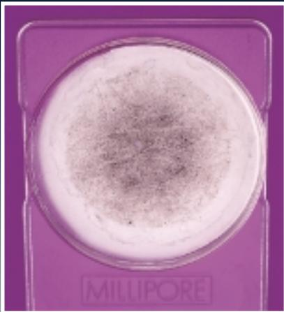
**Trapped.** Potential light-blocking particles from an optical gel were trapped on this 3-micron filter.
