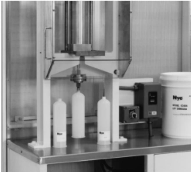
**Clean room, clean grease.** Clean air for a 10-foot mini-environment blankets the working surface, where lubricants are ultrafiltered and packaged in a Class 100 environment.
