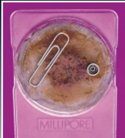
**Long, quiet life.** Contaminates filtered from one pound of bearing grease used in computer applications are displayed next to miniature balls and a bearing. Without ultrafiltration the bearing would have had a short and noisy life. (The paper clip is added for scale)
