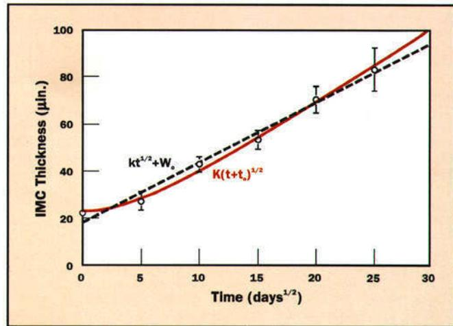
**Figure 13.** IMC growth in HALT over Alloy 521 at 75°C. The curve fits are as indicated on the plot.
