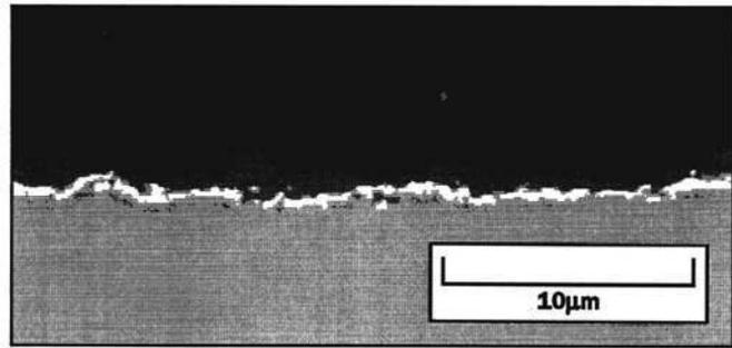
**Figure 1.** BSE SEM image acquired and stored by image analysis system. Inverse of the original gray scale is used. a) tin, b) IMC, c) Alloy 510. Sample was aged at 100°C for 169 days.
