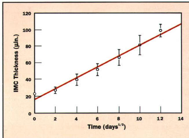
**Figure 11.** IMC growth in HALT over Alloy 510 at 100°C. Averages and standard deviations. Line is a linear fit through the averages.
