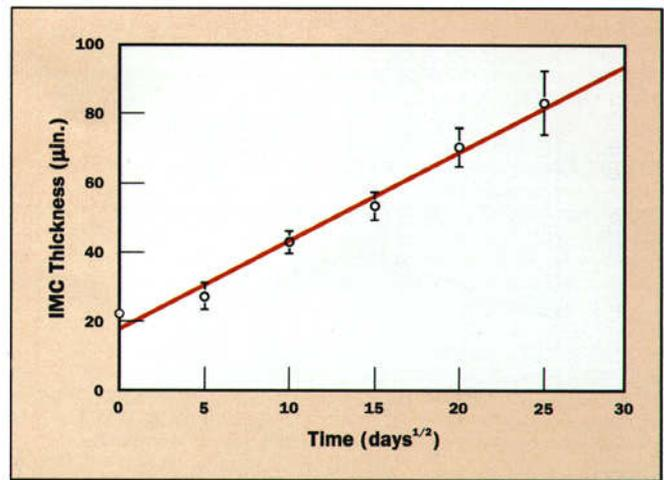
**Figure 7.** IMC growth in HALT over Alloy 521 at 75°C. Averages and standard deviations. Line is a linear fit through the averages.
