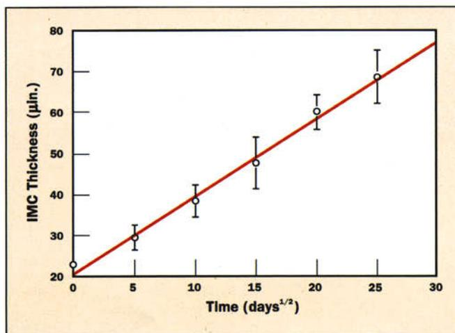
**Figure 10.** IMC growth in HALT over Alloy 510 at 75°C. Averages and standard deviations. Line is a linear fit through the averages.
