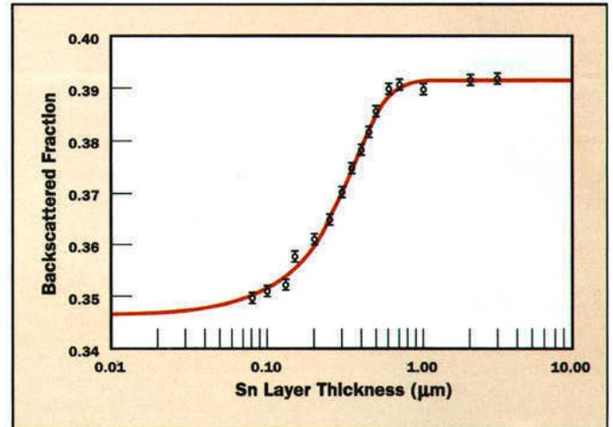
**Figure 4.** Backscattered fraction of the incident electrons at 20 KeV versus the thickness of tin layer over bulk  $\text{Cu}_6\text{Sn}_5$ . Monte Carlo simulation.
