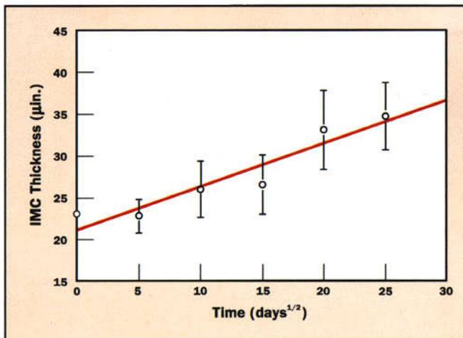
**Figure 9.** IMC growth in HALT over Alloy 510 at 50°C. Averages and standard deviations. Line is a linear fit through the averages.
