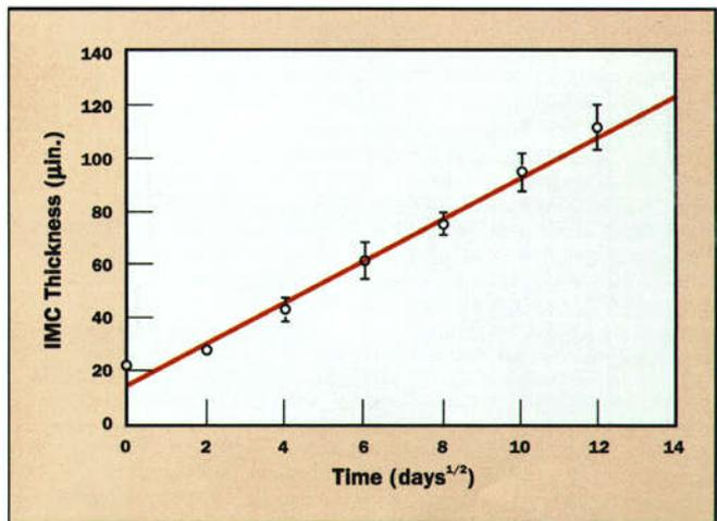
**Figure 8.** IMC growth in HALT over Alloy 521 at 100°C. Averages and standard deviations, Line is a linear fit through the averages.
