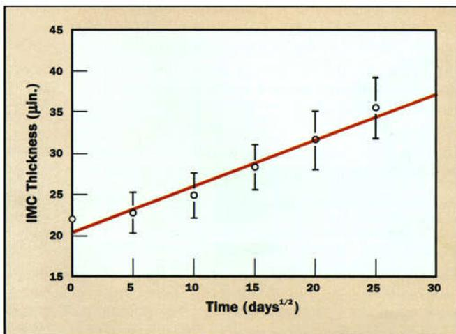
**Figure 6.** IMC growth in HALT over Alloy 521 at 50°C. Averages and standard deviations. Line is a linear fit through the averages.
