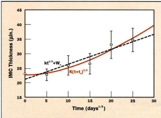
**Figure 15.** IMC growth in HALT over Alloy 510 at 50°C. The curve fits are as indicated on the plot.
