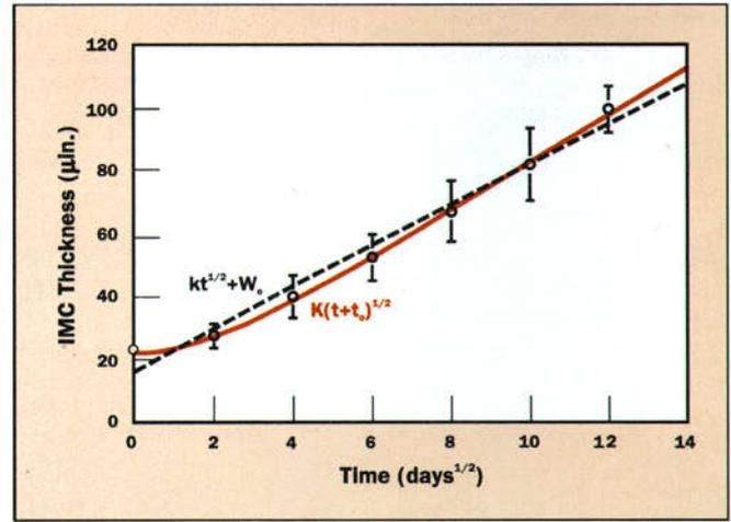
**Figure 17.** IMC growth in HALT over Alloy 510 at 100°C. The curve fits are as indicated on the plot.
