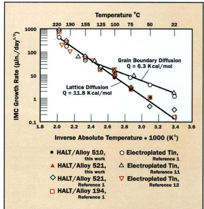
**Figure 18.** True parabolic growth rates for Cu-Sn IMC in various tin coatings. Lines are linear fits through data: for grain-boundary diffusion, electroplated tin from 22°C to 125°C; for lattice diffusion, combined HALT (50°C to 220°C) and electroplated tin (155°C to 220°C).
