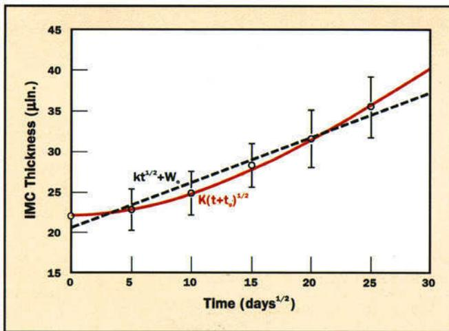
**Figure 12.** IMC growth in HALT over Alloy 521 at 50°C. The curve fits are as indicated on the plot.
