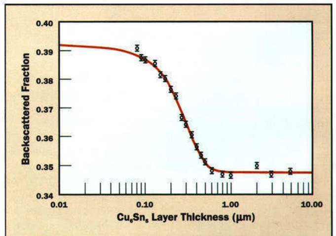
**Figure 5.** Backscattered fraction of the incident electrons at 20 KeV versus the thickness of  $\text{Cu}_6\text{Sn}_5$  layer over bulk tin. Monte Carlo simulation.
