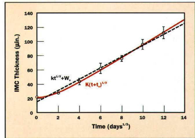
**Figure 14.** IMC growth in HALT over Alloy 521 at 100°C. The curve fits are as indicated on the plot.
