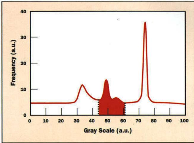
**Figure 2.** Gray-level diagram of the image in Figure 1. Two peaks in the middle correspond to IMC. Shaded area represents the ROI on the scale.
