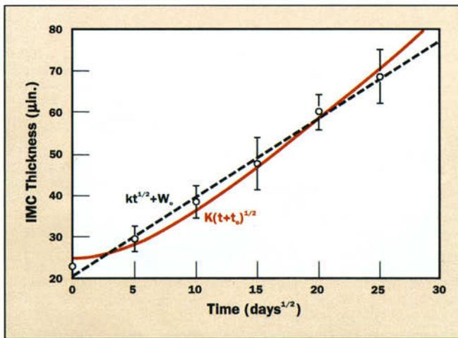
**Figure 16.** IMC growth in HALT over Alloy 510 at 75°C. The curve fits are as indicated on the plot.
