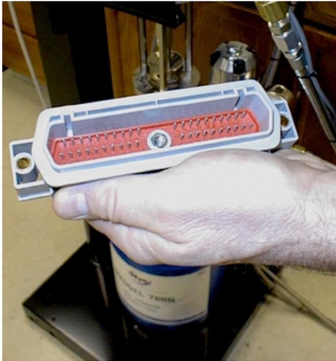
**Figure 3: Dispensing the Grease** This semi-automatic connector grease dispensing system, custom designed by LCC/Dispensit of Indianapolis, Ind., allows the operator to dispense minute amounts of grease in multiple locations simultaneously, quickly, and precisely.
